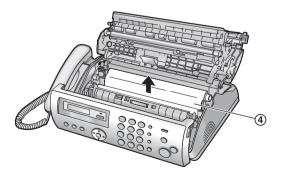
4 Clean the thermal head (⑤) with a cloth moistened with isopropyl rubbing alcohol, and let it dry thoroughly.
